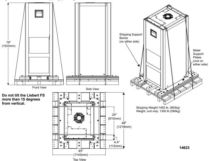
The FS as shipped (see **Figure 8**) can weigh up to 1,462 lb. (663kg). It must be handled with care. It must be kept upright—pay special attention to the arrows, which indicate the upright position.
